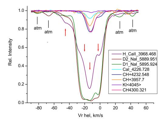
Puc. 1: Figure 1. Profiles of interstellar lines obtained from the 6-meter telescope Cyg X-1 optical spectra: relative intensity vs heliocentric radial velocity  $V_{r\ hel}$ . Profiles are shown by different colors according to the imbedded panel. Black ticks labeled "atm" mark positions of the terrestrial atmosphere  $H_2$  absorption lines on the D1 and D2 Na I line profiles. Red arrows indicate radial velocities of the main components of the interstellar line profiles.
